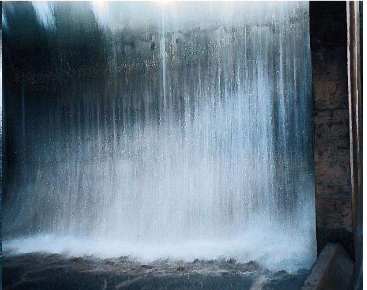
Tipping Buckets Dropping Water Load at 2000 gals/bucket
