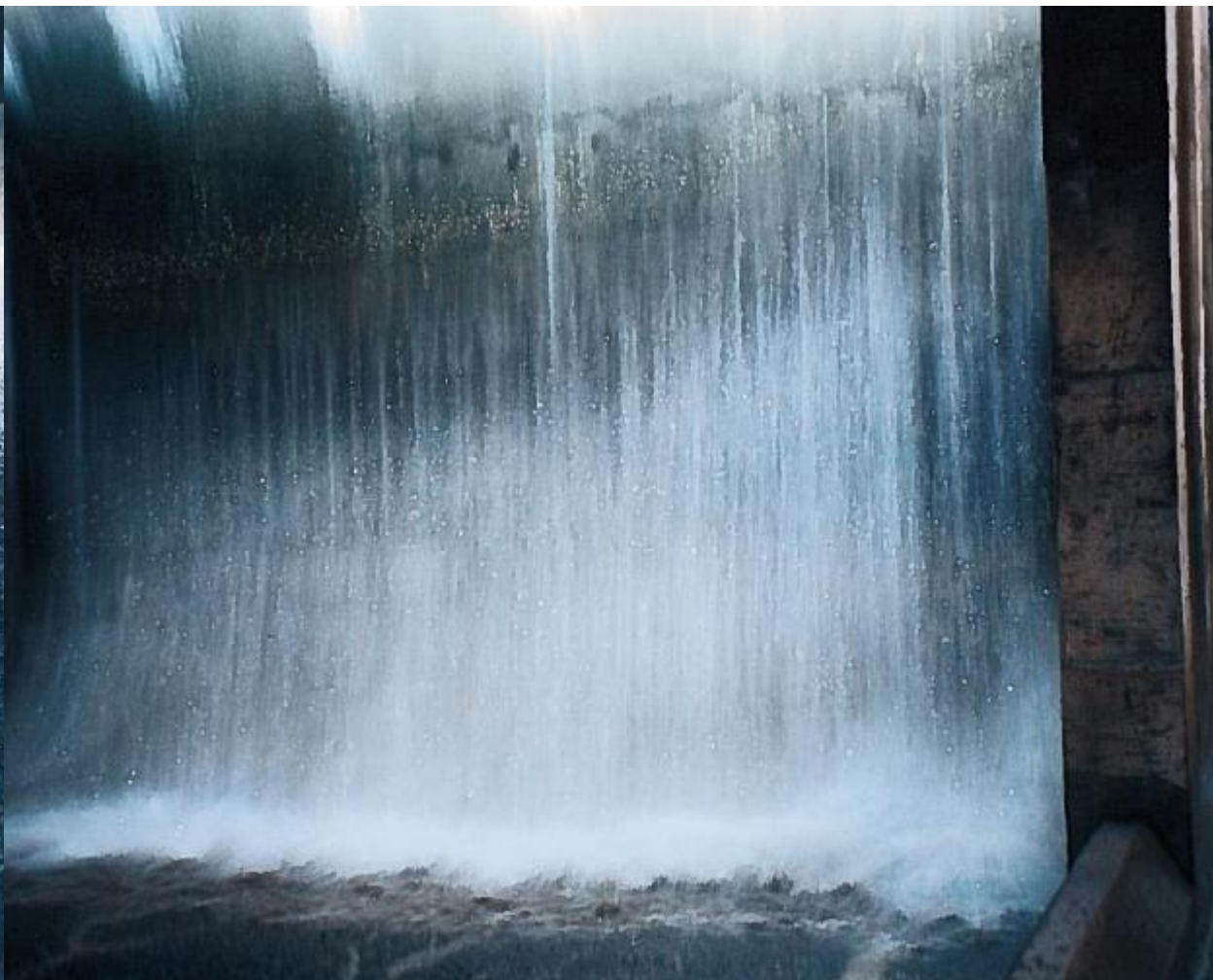
Tipping Buckets Dropping Water Load at 2000 gals/bucket
